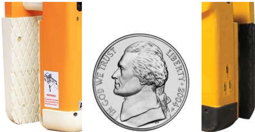
Place a **NICKEL** head first into several tread grooves across the **rubber plate**. **If you** always see the top of Jefferson's head, **your** rubber is too shallow and worn. **If this is the case, REPLACE EITHER CENTER PLATE OR BACK PLATE** or both. **If** part of Jefferson's head is always covered by the Rubber wall of the plate you are inspecting, **you** have enough rubber depth remaining.
